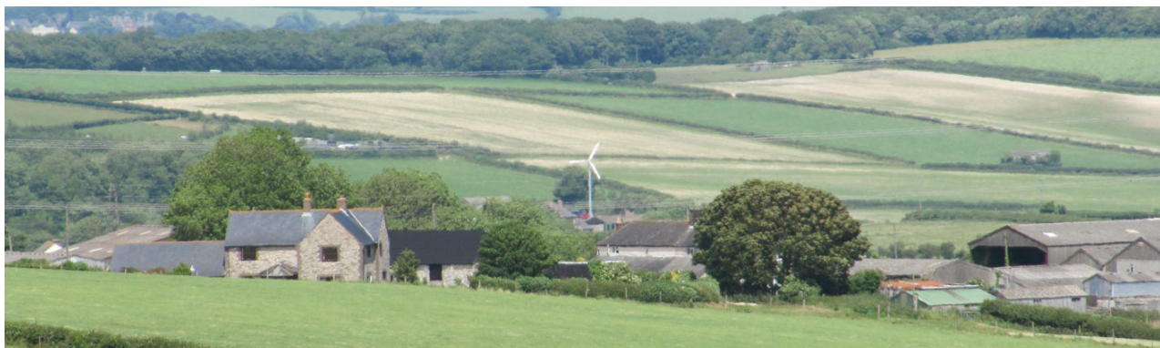
Photo 1: Rew Manor Farm, West Dorset, chalk downland landscape (Planning application ref: 1/D/09/001280 1 ) Scale & siting: 12m to hub / 16m to blade tip. A well sited small scale turbine, grouped with existing development, within the trough of the landform and well below the skyline.
